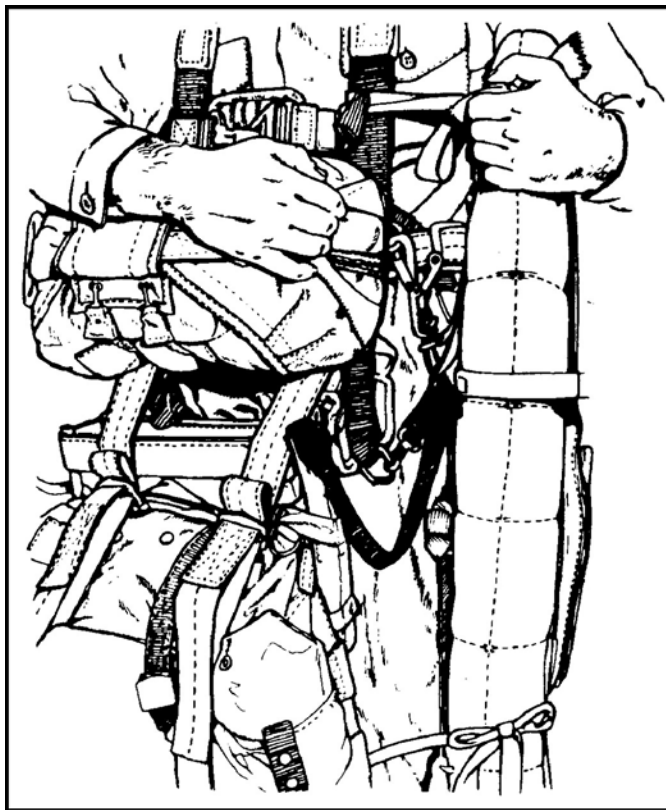
Figure 12-8. Lowering line attached for tandem rigging.
